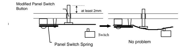
The part number for the new Panel Switch Spring Plate is P000227690. The part number for the modified Panel Switch Button is P000227080; however, the current button can be modified by simply removing the pin at the bottom of the button. The new parts will not be available for a few weeks.
