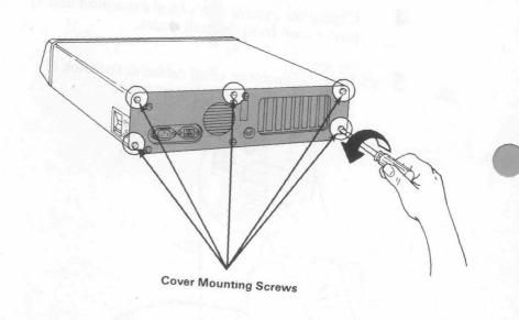
Carefully slide the unit's cover away from the rear and to the front, as shown in the figure rear and to the cover will go no farther, tilt it below. When the cover will go no farther, tilt it up, remove it from the base, and set it aside.
