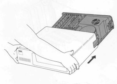
When the cover is all the way to the rear, align the screws with the threaded tabs and tighten. Use a flat-blade screwdriver or 1/4-inch nutdriver and turn clockwise.
