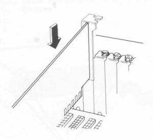
Align the slot in the adapter retaining bracket with the hole in the rear panel of the unit. Start the screw clockwise, then tighten with a flat-blade screwdriver or 3/16-inch nutdriver.
