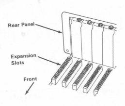
11 Use a flat-blade screwdriver or 3/16-inch nutdriver and remove the screw that holds the expansion slot's cover in place by turning the screw counterclockwise. Save the screw for the installation of the option. Remove the expansion slot's cover.
