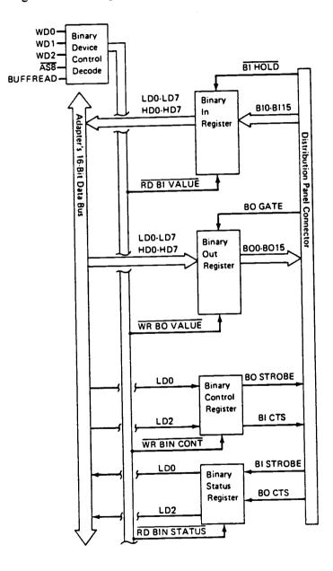
The Data Acquisition Adapter's binary I/O device has the following features:
